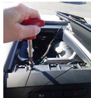
Screws to remove radio bezel
