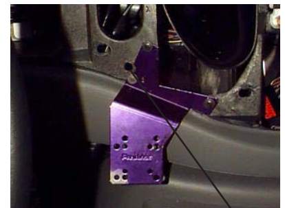
Do not cover this hole. InDash placement and screw locations.
