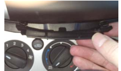
Removal of Cover Strip
