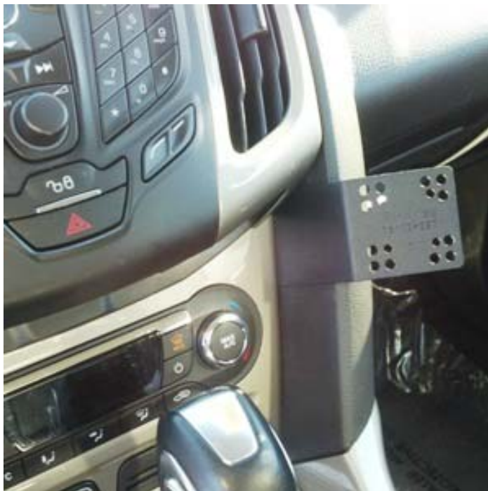
InDash installed showing finished install location
