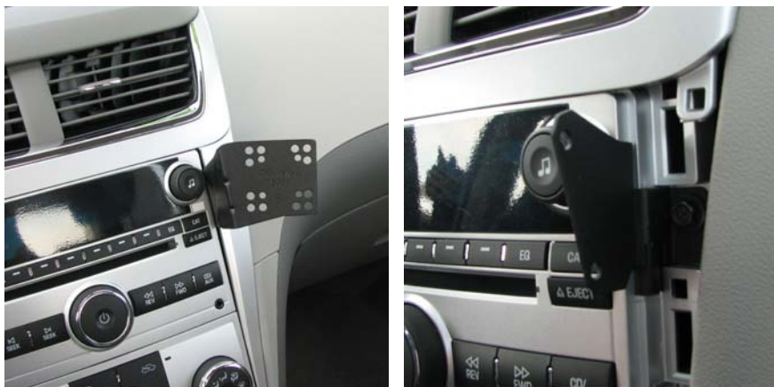
Installation of InDash Mount
