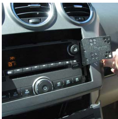
Installation of InDash Mount
