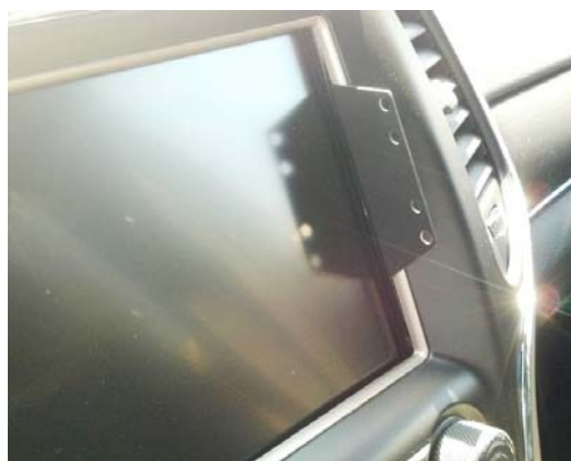
Bottom part of InDash Mount installed w/Display
