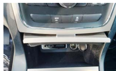
Open Cubby door and pull from bottom of bezel under switches
