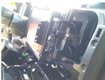
InDash mount bottom installed showing screw location and mount
