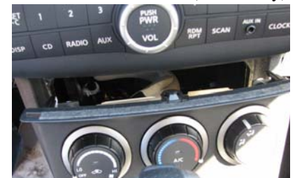
Climate Control Removal (All)
