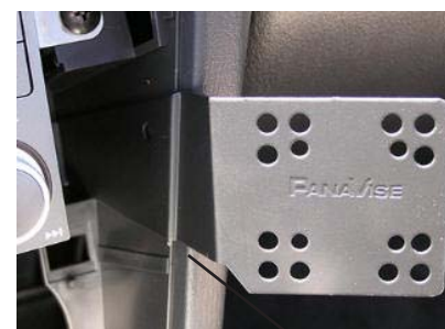
InDash installed showing alignment of joggles
