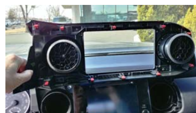
Radio bezel removal showing (10) clips for removal of radio bezel.
