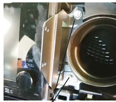
InDash showing (2) mounting bolts placement.
