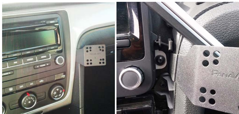
InDash installed showing mounting location
